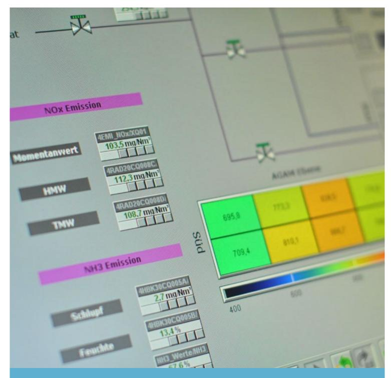
**Environmental Technology** SNCR control system by SAR
